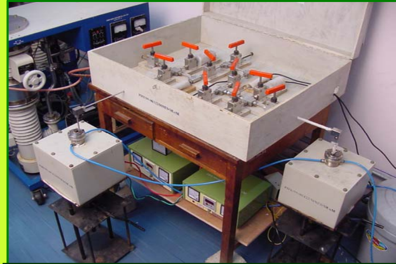
Hydrogen absorption units
