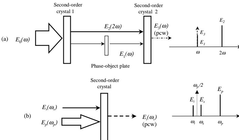
Fig. 10. Three-wave mixing for generating forward PCW in a second-order nonlinear crystal: (a) degenerate difference-frequency generation, (b) quasi-degenerate difference-frequency generation.
