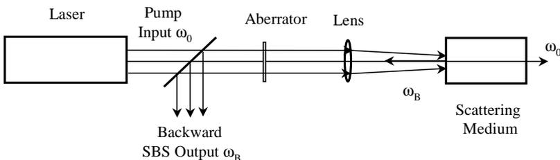
Fig. 17. Experimental arrangement for observing phase-conjugation behavior of backward stimulated Brillouin scattering.
