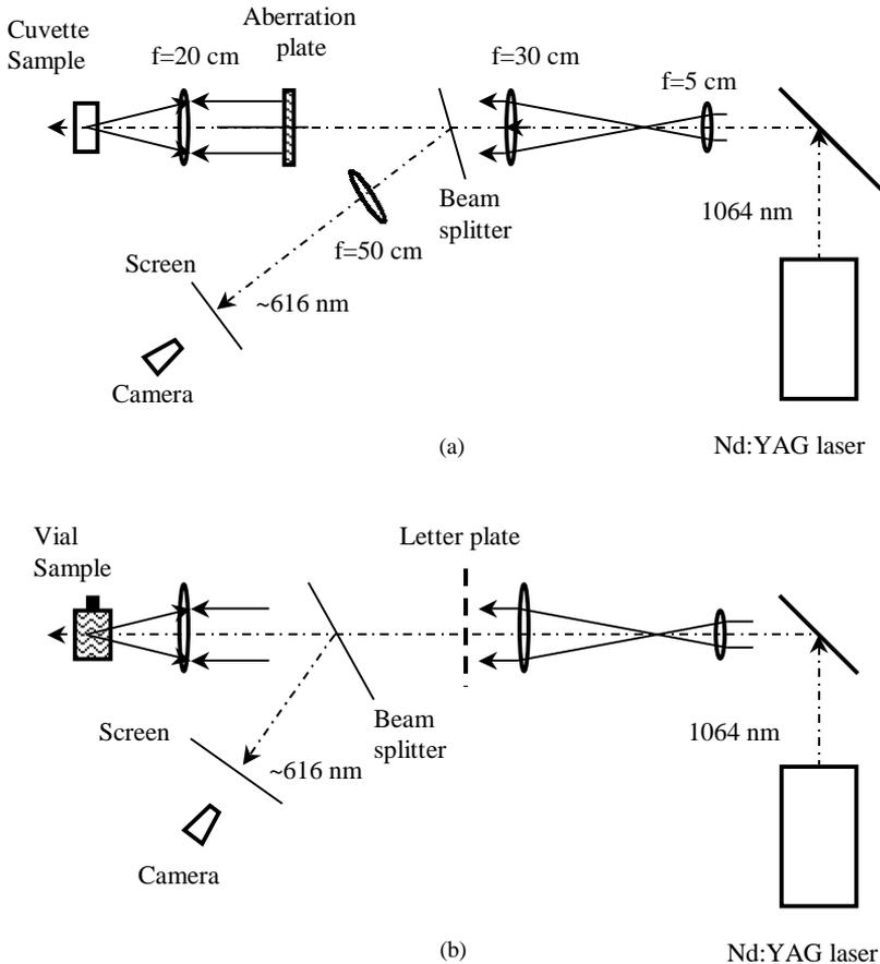
Fig. 23. Experiment for demonstrating phase-conjugation properties of the TPP backward stimulated emission: (a) configuration for the far-field measurement and (b) configuration for the near-field image measurement.
