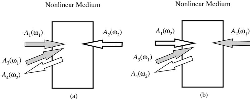
Fig. 7. Schematics describing the generation of the backward nondegenerate PCW via partially degenerate FWM in a nonlinear medium.
