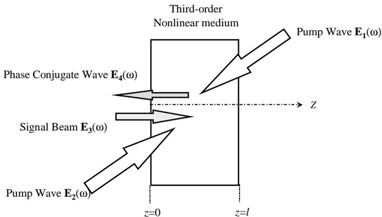
Fig. 4. Phase-conjugate wave generation by degenerate four-wave mixing.
