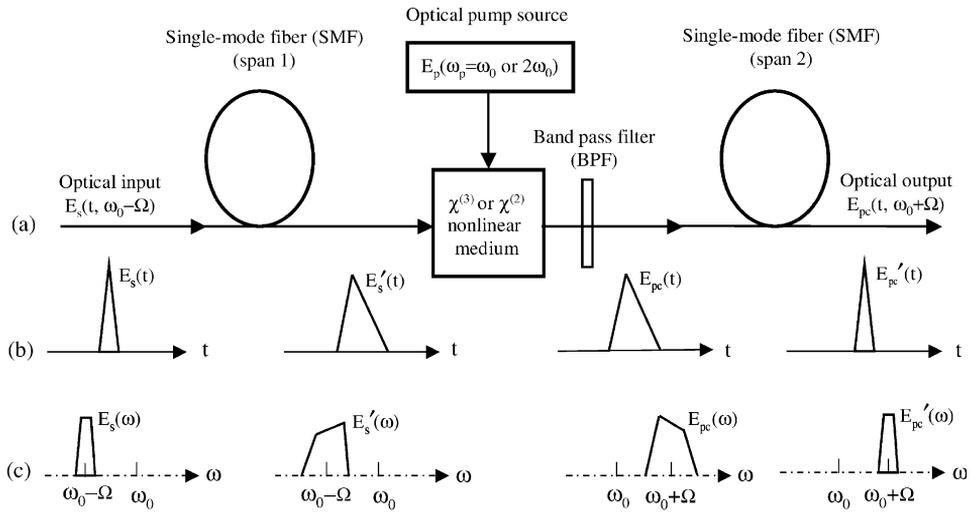
Fig. 30. (a) Schematic diagram showing midway optical phase conjugation (mid-span spectral inversion) between two long spans of single-mode fibers, (b) waveform changes of the input signal pulse and output phase-conjugate pulse, (c) spectrum changes of the input signal pulses and output phase-conjugate pulse.
