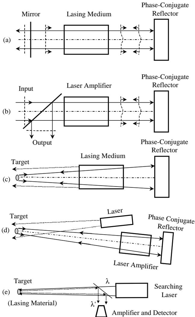
Fig. 29. (a) High-brightness laser oscillator with a phase conjugate reflector as the rear cavity-reflector, (b) high-brightness two-pass laser amplifier with a phase conjugate reflector, (c) laser target-aiming and auto-focusing system, (d) laser target-aiming and weapon system, (e) laser identification and rescue system.
