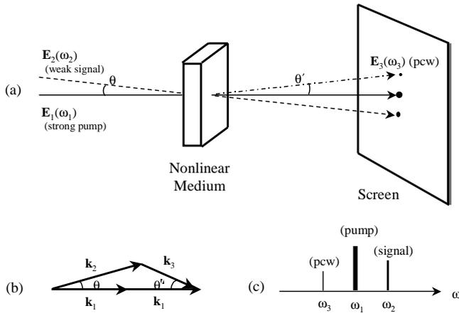
Fig. 9. Forward nondegenerate FWM for generating forward PCW: (a) optical layout, (b) phase-matching, and (c) spectral locations.
