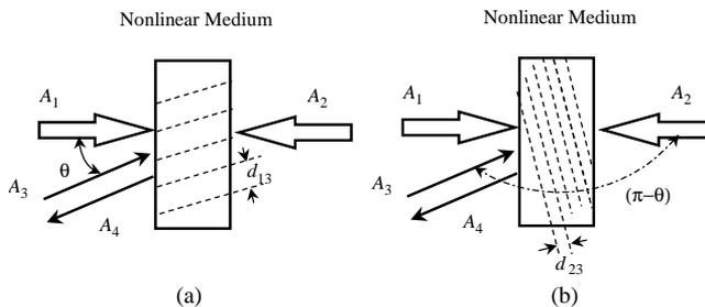
Fig. 5. Schematics describing the generation of a backward phase conjugate wave via induced holographic gratings.
