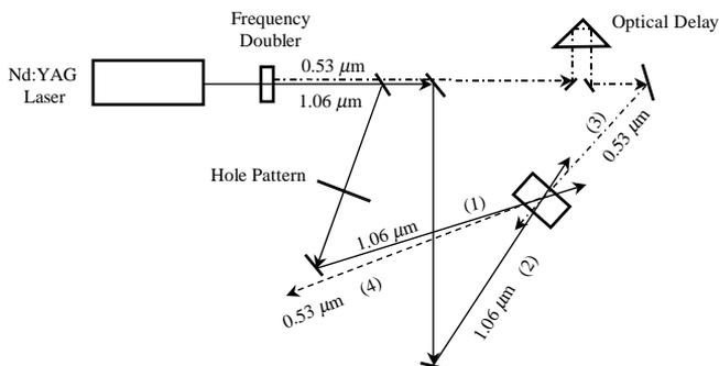
Fig. 14. Optical layout for generating PCW via nondegenerate FWM.
