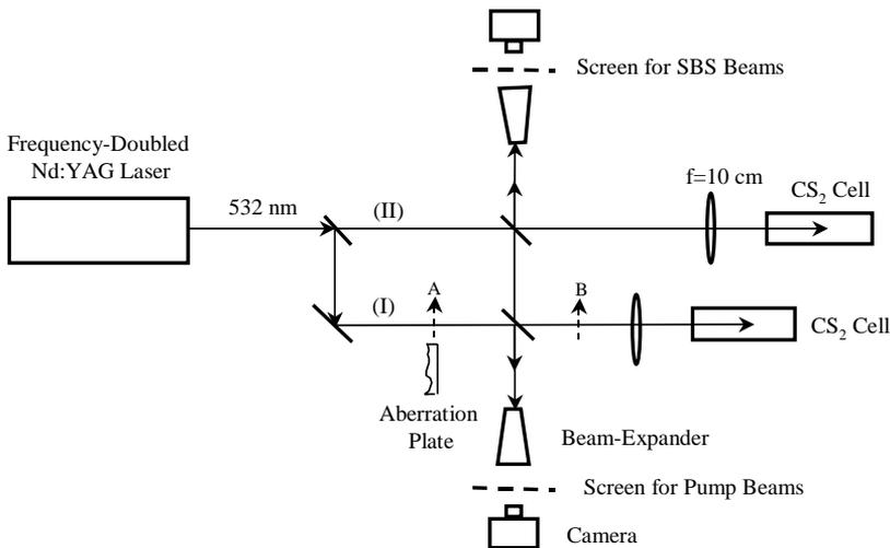
Fig. 20. Experiment for examining the wave-front reconstruction property of backward SBS by two-beam interference method. The aberrator can be inserted in position A or B of the optical path (I). (From Ref. [32].)
