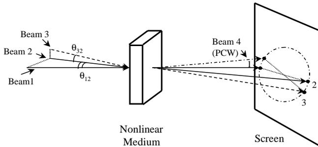
Fig. 8. Forward degenerate FWM setup for generating forward PCW.
