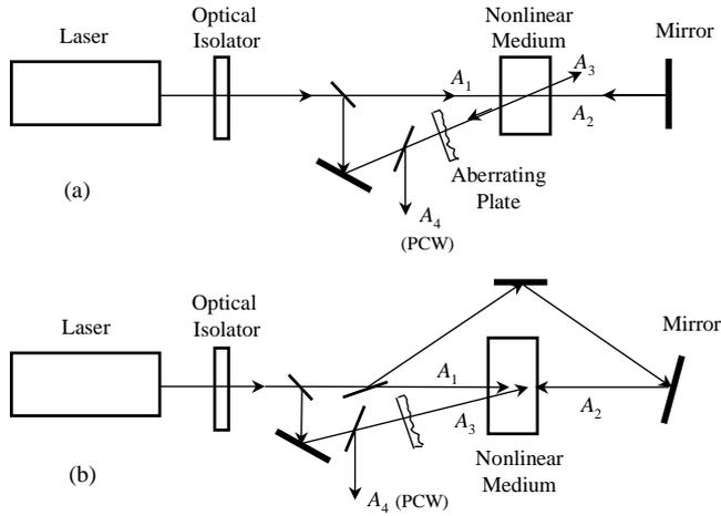
Fig. 11. Two typical experimental setups for PCW generation via degenerate four-wave mixing.
