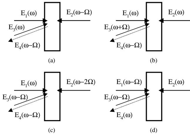
Fig. 16. Brillouin-enhanced FWM with different frequency-combinations for generating PCW with a frequency downshifted (a) and (b), unshifted (c), and upshifted (d).
