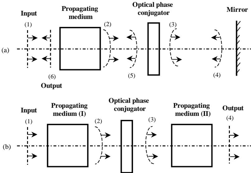
Fig. 3. Forward PCW generation and phase-distortion correction: (a) the combination of an optical phase conjugator with an ordinary mirror reflector; (b) the optical phase conjugator is placed in the middle of two identical propagating systems.
