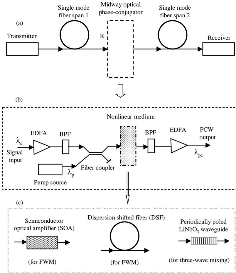
Fig. 31. (a) Midway optical phase conjugation (MOPC) employed in long transmission distance and high bit-rate optical fiber communication systems, (b) basic components of a midway optical phase-conjugator, (c) three types of nonlinear media for MOPC purposes. BPF: band-pass filter; EDFA: erbium-doped fiber amplifier; FWM: four-wave mixing; PCW: phase-conjugate wave.
